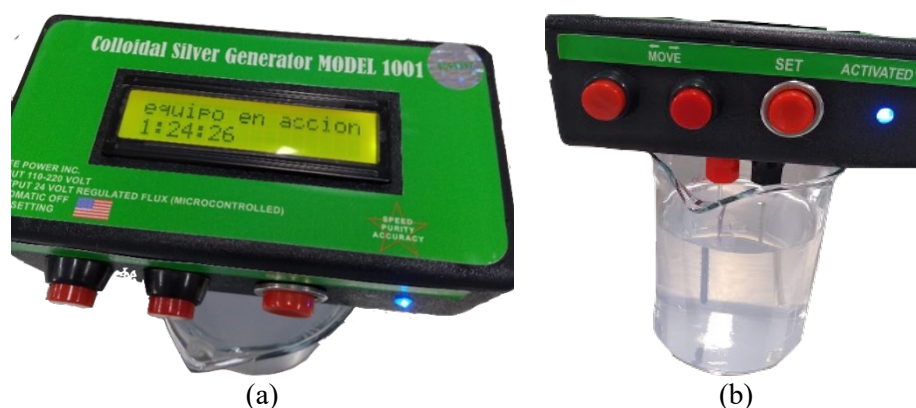
Figure 1. Silver Generator® model 1001 colloidal system, used for the synthesis of AgNPs at room temperature. (a) Colloidal silver generator model 1001; (b) Silver nanoparticle solution.
