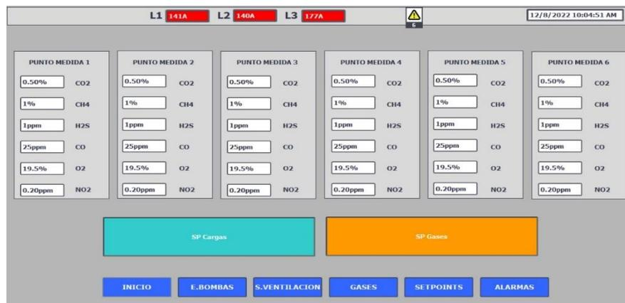
**Figura 41. Setpoints de gases**
