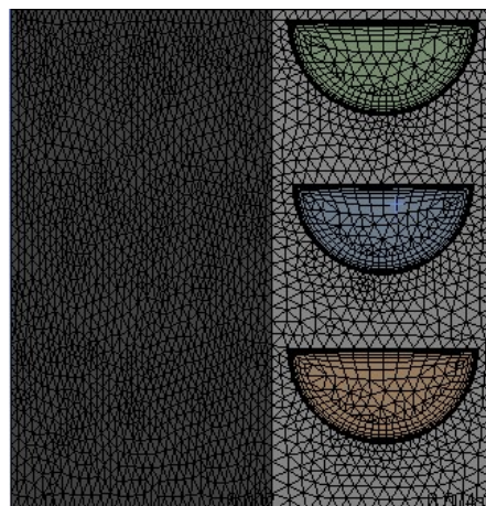
Figure 4. The structured mesh of the computational domain.
