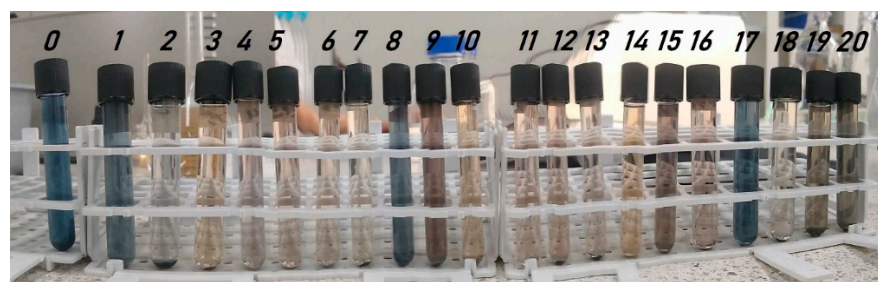
Figure 1. Dyeing wastewater samples before (0) and after treatment (1–20) (0–20 from left to right).
