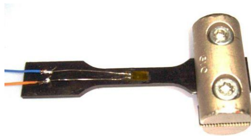
Figure 4. PA6 specimen reinforced with strain gauge for impact traction.
