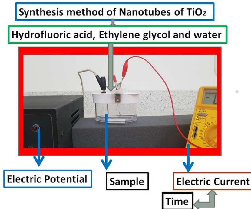
**Figure 1.** Experimental procedure for obtaining nanotubes from the titanium sheet.
