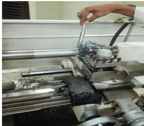
Figure 3. Machining of specimens for honing tool testing.
