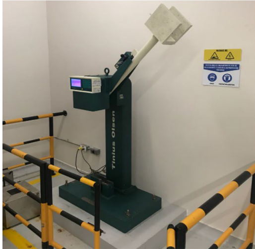
Figure 1 Impact test machine type Charpy
