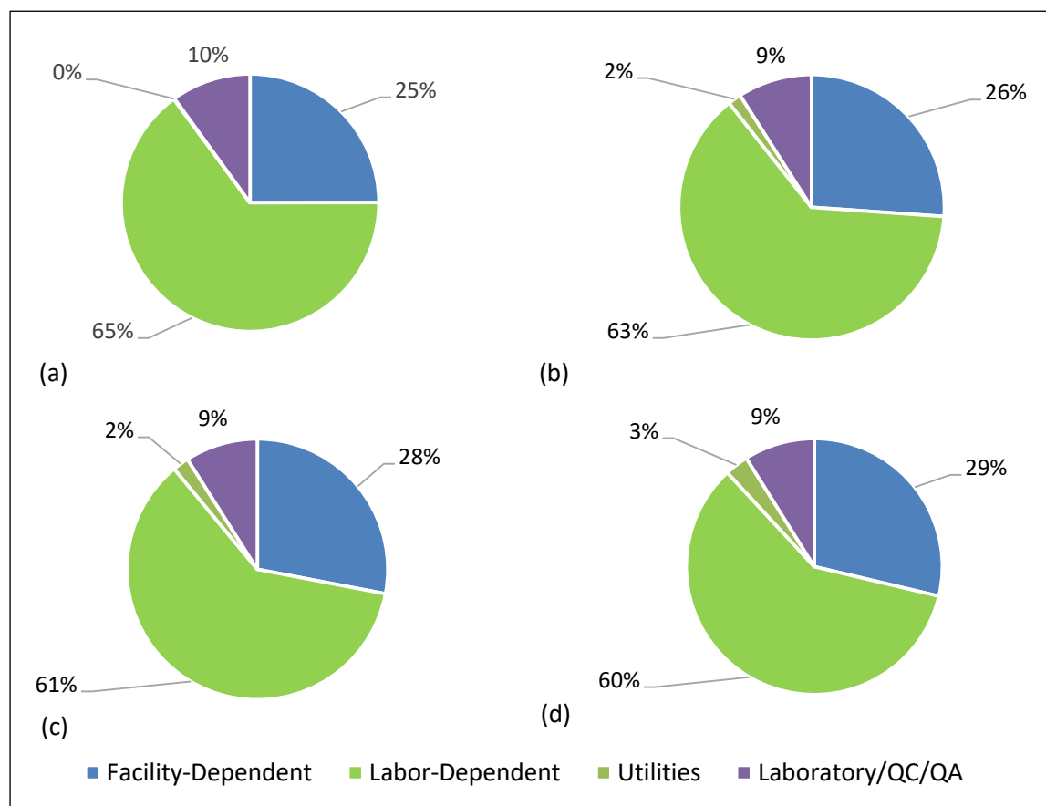
Figure 4. Annual Operating cost estimations for Chlorella large scale production based on mass flow effect: (a) 20 kg/h, (b) 60 kg/h, (c) 100 kg/h and (d) 140 kg/h.
