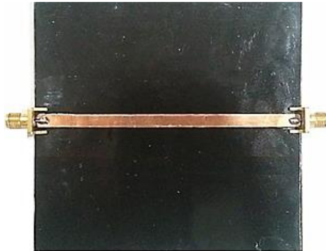
Figure 3. Configuration of the microstrip transmission line.
