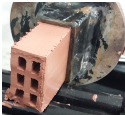
Figure 3. Extrusion process of H10 block in laboratory scale.
