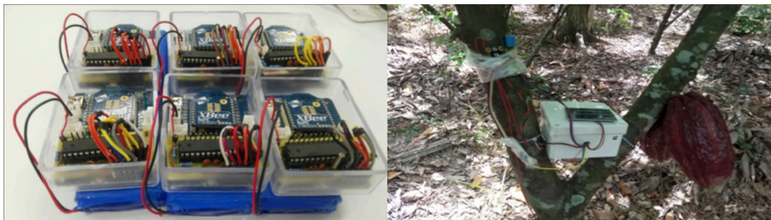
Figure 3. a) 6 Zigbee wireless sensor nodes. b) Zigbee wireless sensor node on the cocoa crop.
