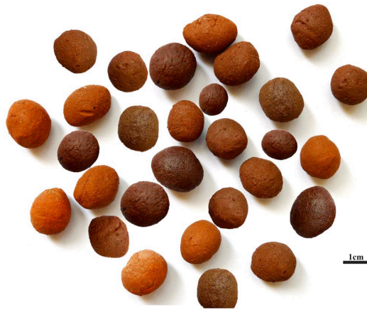
Figure 1. Clay expanded in the production process of light aggregates.
