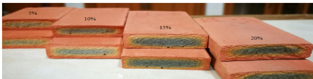
Figure 4. Photographic record of ceramic samples made using the unburned bodies (wastes).
