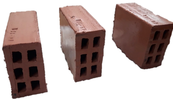
Figure 3. H10 blocks manufactured at laboratory scale in the CIMAC. Wet condition in M CRHb-5.
