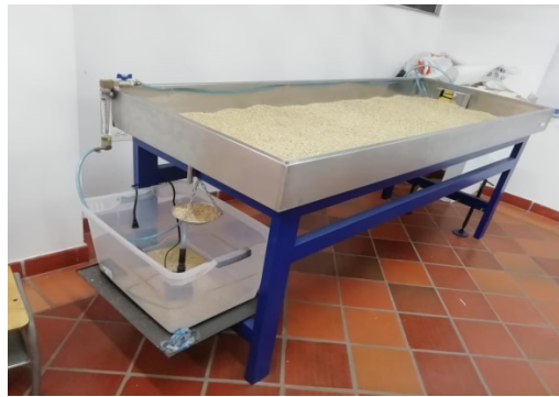
Figure 1. View of the river simulator used.
