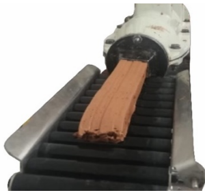
Figure 1. Eco Design laboratory scale extrusion.
