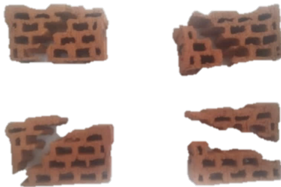
Figure 4. Samples after compression resistance test.
