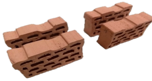
Figure 2. Eco Design prototypes manufactured in M CRH-5 at laboratory scale.
