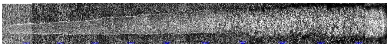
Fig. 12. Scoring footprint for coatings {Bi-Ti/20-80} in Bilayer at 1500 rpm.
